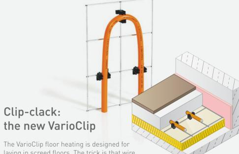
laying in screed floors. The trick is that wire mesh is simply laid on, and the VarioProFile pipe locks easily into the holding clips provided. This is really quick to do and keeps the pipe stable at the perfect distance.
