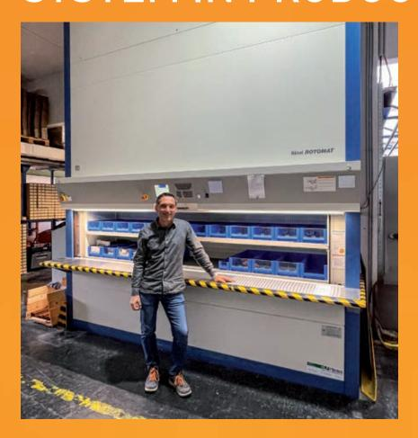
The new carousel, which is affectionately known internally as a paternoster, offers a remarkable 48m² of storage space on a 15 m² footprint. Around 800 spare parts - naturally provided with master data and article numbers - find their allocated space and enable smooth maintenance and repairs of our special machines. "This further important digitalisation step now ensures smooth maintenance processes," says a delighted Gernot Baumgartner, our Head of Production.
